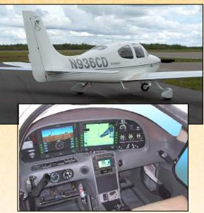
Powerplant Gross Weight Cruise Speed Instrumentation TCM IO-360ES 200 HP 3000 Ibs 150 KTAS VFR
