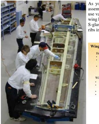
As you can see in the photo to the left that assembly is very labor intensive, and they also use vacuum bagging to make the skins for each wing half. The ribs in this photo are made out of S-glass, but they have reduced the number of ribs in the G-3 series aircraft depicted below:
