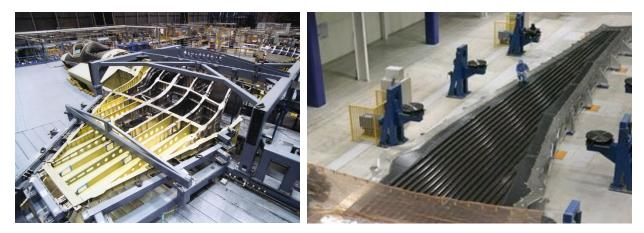
As each section is created it is ready to be moved or integrated into the next piece. If wing longerons are made as in the right image, depth of the robot creates layers in the upper half of the wing and tensioned between the initial layers forming a flexible wing but with high wing loading.
